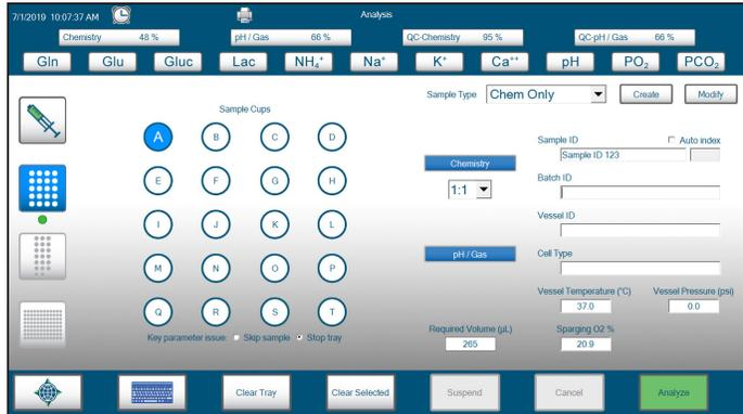
**CAUTION:** *Nova recommends that Sample Cup and Eppendorf tubes be filled with 400 $\mu$ L to mitigate short sampling. For Sample Cup analysis, use the Bioprofile Sample Cup (PN 58275).*
