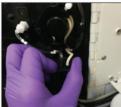
4.21 Disconnect Tubing Manifold
