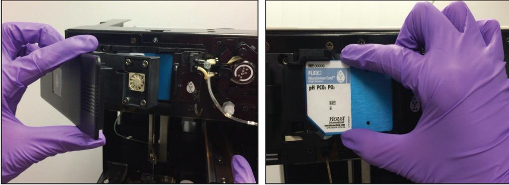
4.11 Open Sensor Module Door and Remove Old and Install New Sensor Card
