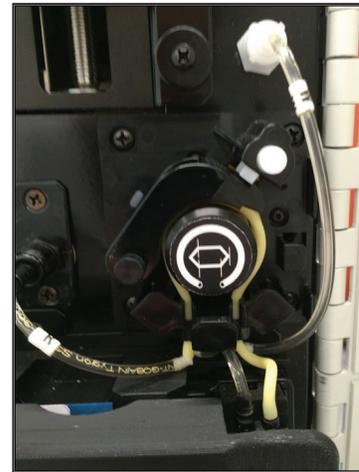
3.9 Chemistry Pump and Pump Tubing Harness
