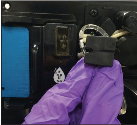
4.13 Disconnect Tubing Manifold
