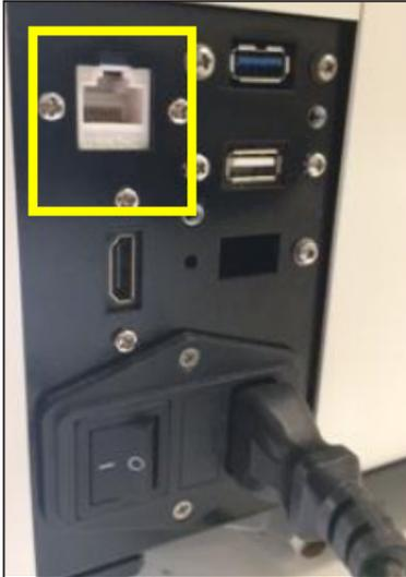
3.25 Ethernet Port for Network Cable from LAN
