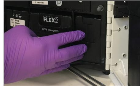
3.15 pH/Gas Auto QC Cartridge Flush with Chassis
