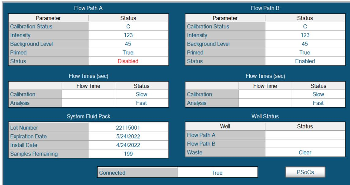
Figure 1.8 System Fluid Screen
