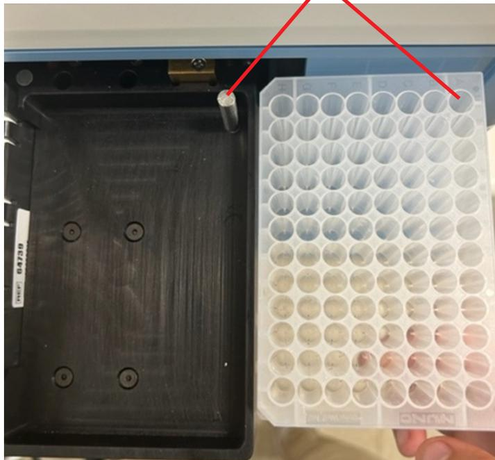
Figure 3.6 96-Well Plate Positioning in Drawer
