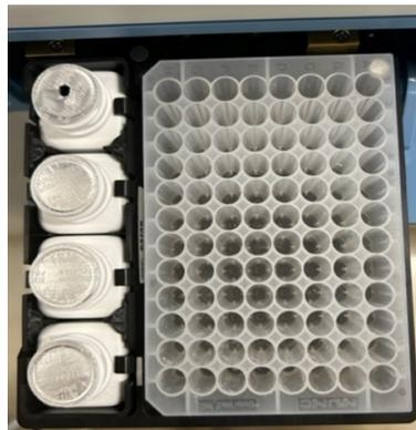
Figure 4.6 Correct Orientation of the 96-Well Plate
