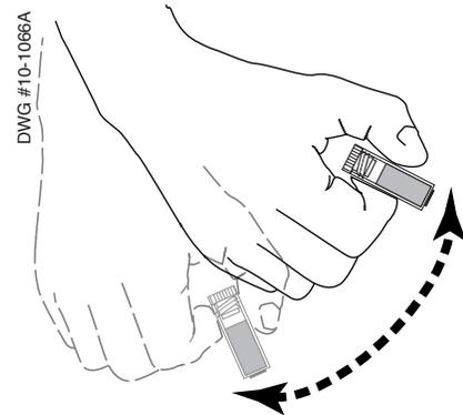
Figure 4.2 Shaking Down Membrane Cap
