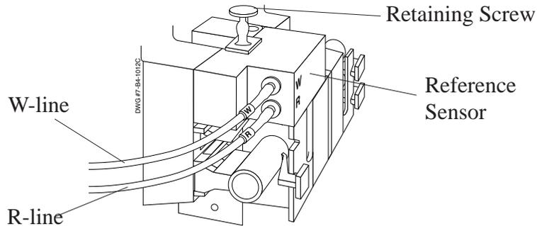
Figure 4.6 Disconnecting the Reference Electrode
