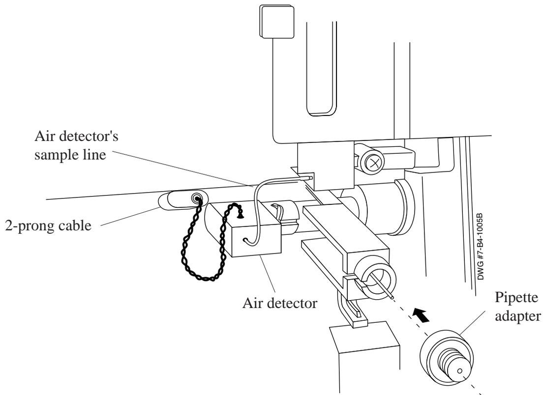
Figure 4.13 Removing Pipette Adapter
