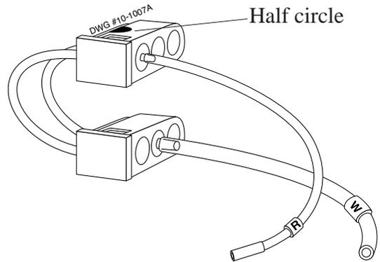
Figure 4.8 Pump Tubing
