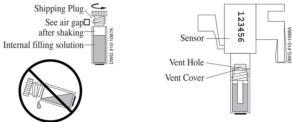
Figure 4.3 The PCO<sub>2</sub> Membrane Cap (With Shipping Plug and Attached to Sensor)
