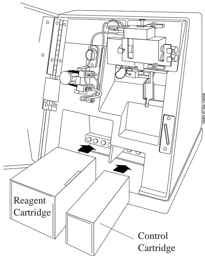
Figure 4.1 Replacing the Reagent Cartridge and the Control Cartridge
