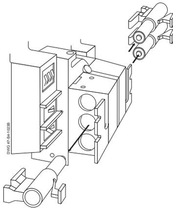
Figure 4.15 Removing the Sensors
