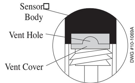
Figure 4.4 Vent Cover on Membrane Cap
