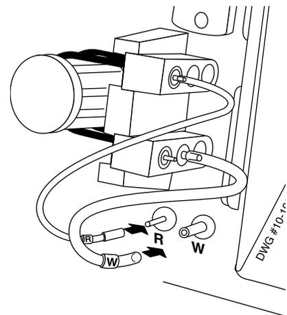
Figure 4.9 Connecting the Pump Tubing W and R-lines
