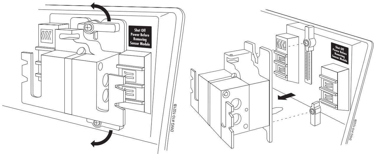
Figure 4.16 Unlocking and Removing the Sensor Module
