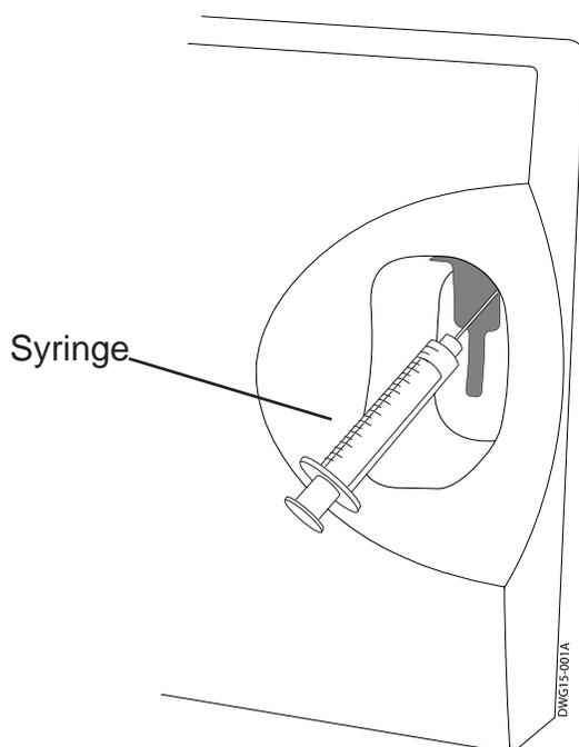
Figure 3.3 Analyzing from a Syringe
