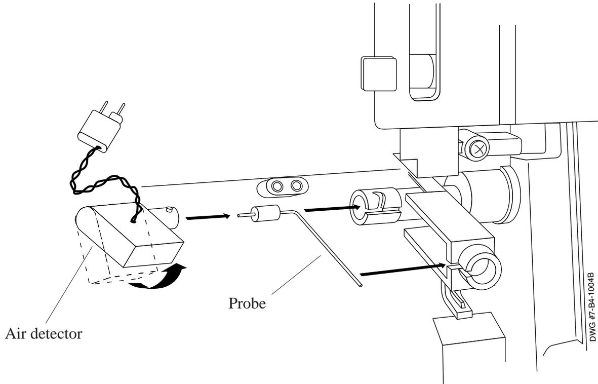
Figure 4.14 Replacing Probe and Air Detector
