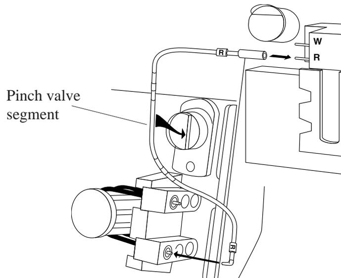
Figure 4.11 Connecting the R-line
