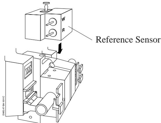
Figure 4.7 Placing New Reference Electrode onto Sensor module
