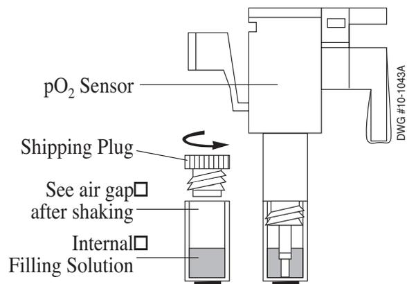
Figure 4.5 Installing the PO<sub>2</sub> Membrane Cap
