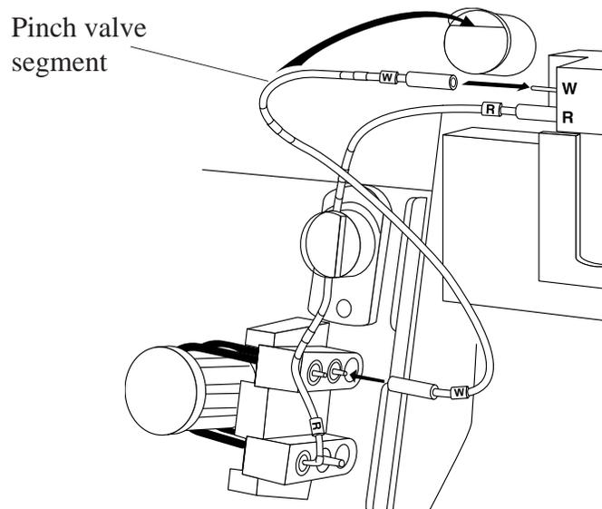
Figure 4.10 Connecting the W-line
