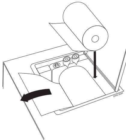
Figure 4.12 Replacing the Printer Paper
