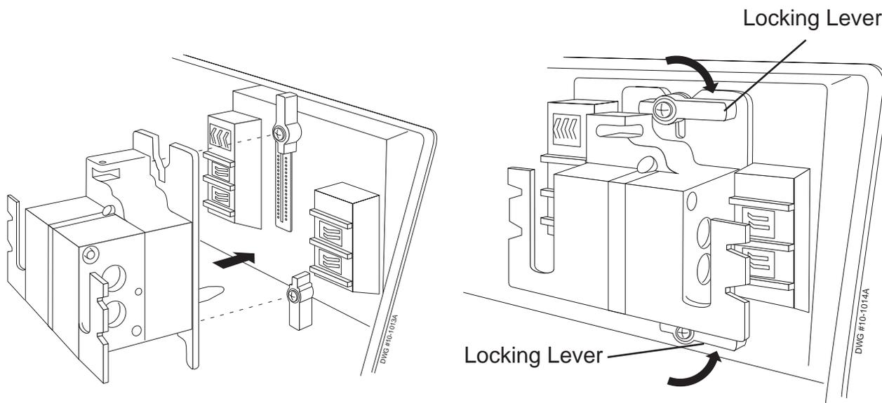
Figure 4.17 Replacing and Locking the Sensor Module
