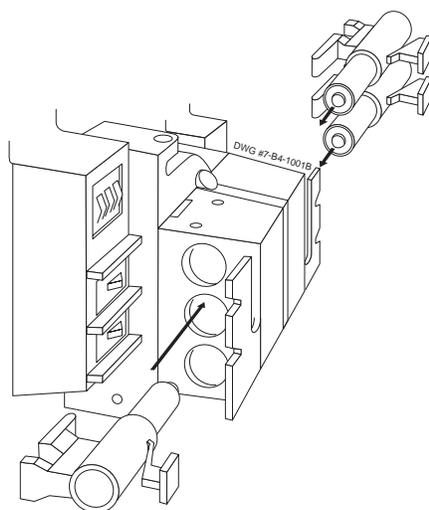
Figure 4.18 Replacing the Sensors
