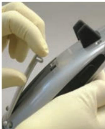
3. Push up on the battery latch. Remove the drained battery.
