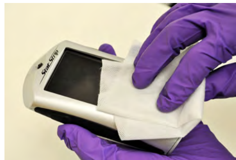
Figure 6.6 Wiping the Surface of the Meter
