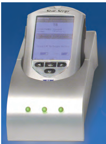
Figure 6.2 Meter placed into Charging Station
