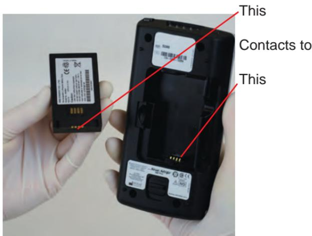
Figure 6.5 Replacing with a Fully Charged Battery
