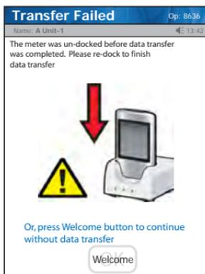
Figure 7.8 Transfer Failed - Transfer Incomplete
