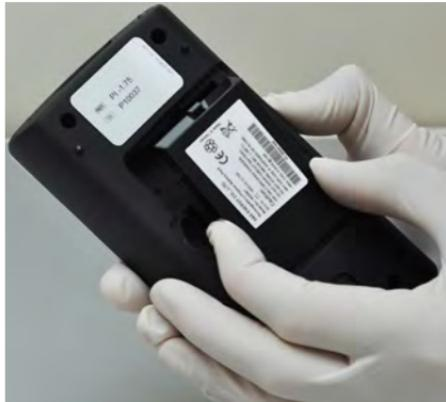
Figure 6.4 Removing the Battery
