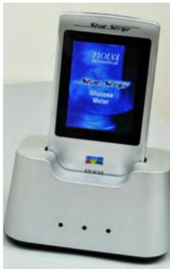
Figure 6.2 Meter placed into Charging Station
