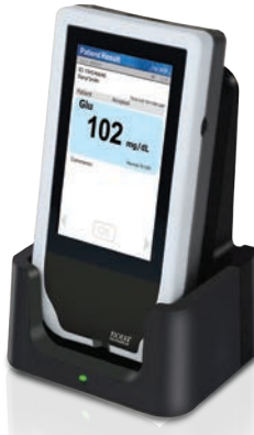
Figure 5.2 Meter placed into Charging Station
