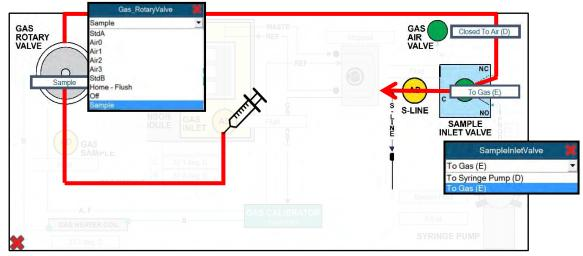
5.3 Sample Inlet Valve and Gas Rotary Valve Menus
