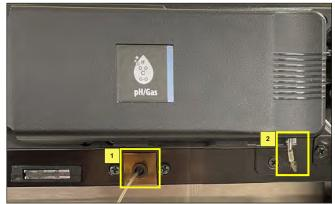
**<sup>5.4</sup>** Unscrew the S-Line Tubing (1) and Disconnect the pH/Gas Sample Inlet Tubing (2)
