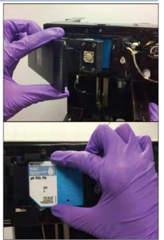
4.12 Open Sensor Module Door and Install New Sensor Card
