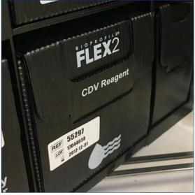
4.33 Pack Flush with Analyzer Chassis
