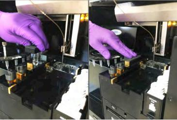
**4.27** Installing and Seating Chemistry Auto QC Cartridge
