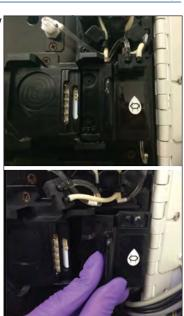
**4.25** Remove Sensor Card & Reference Sensor
