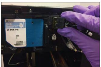
4.7 Disconnect Pump Tubing Manifold
