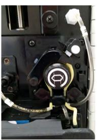
**3.11** Chemistry Pump and Pump Tubing Harness
