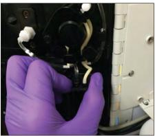
4.24 Disconnect Tubing Manifold
