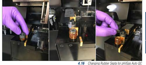
3. Invert the cartridge a few times. Then insert the cartridge into its respective port, and ensure the needle fitments pierce the rubber fitments at the back of the cartridge. The cartridge should be flush with the chassis.
