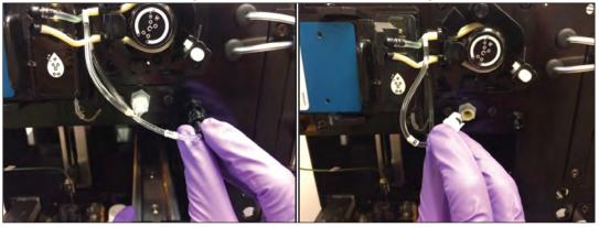
4.8 Waste Tubing Fitting (L) and Reference Tubing Fitting (R)
