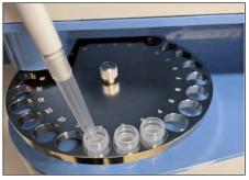
3.73 Pipet Sample into Each Sample Cup
