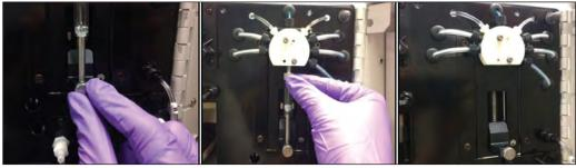
**4.3** Syringe Barrel & Plunger Removal
