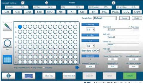
2.26 Microtiter Plate Sample Analysis Screen
