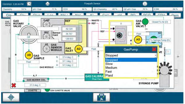
4.43 Gas Module Peristaltic Pump Control
