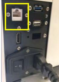
2.55 Ethernet Port for Network Cable from LAN
