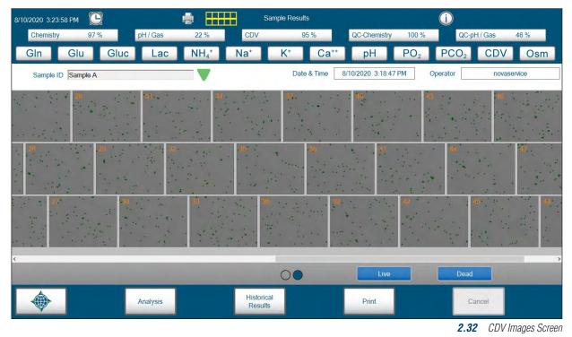
All of the CDV images populated may not fit in the field of view. A slide bar at the bottom of the image tiles allows the operator to slide left and right to see all of the images populated. Select **Live** or **Dead** below the image tiles to turn on the Live and Dead cell indicators:
