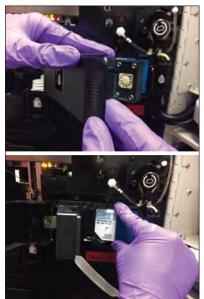
4.22 Open the Chemistry Sensor Module Door and Install New Sensor Card
