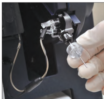
Figure 6.6 Remove Capillary Adaptor
