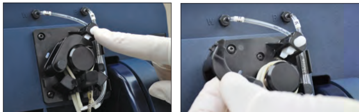
Figure 6.3 Release Pump Tubing Pressure Plate
