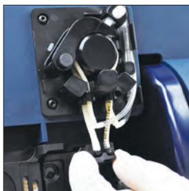
Figure 6.4 Disconnect Pump Manifold
