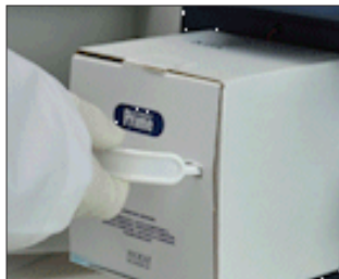
Figure 5.3 Remove Calibrator Cartridge and Capillary Adaptor
