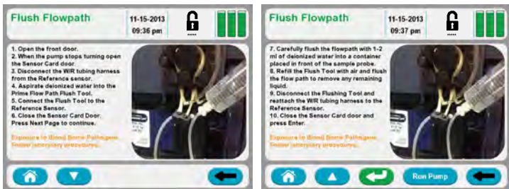
Figure 7.4 Flush Flow Path Screens
