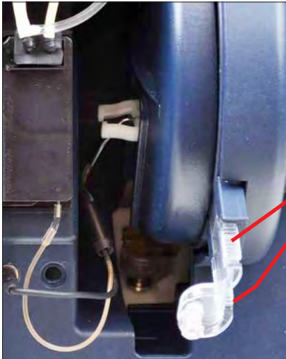
Figure 6.13 Replace the Safety Sample Port
