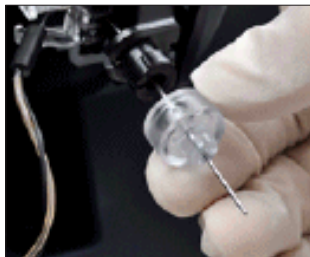
Figure 5.3 Remove Calibrator Cartridge and Capillary Adaptor
