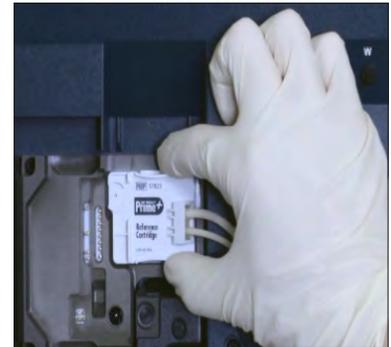
Figure 5.13 Remove Reference Cartridge
