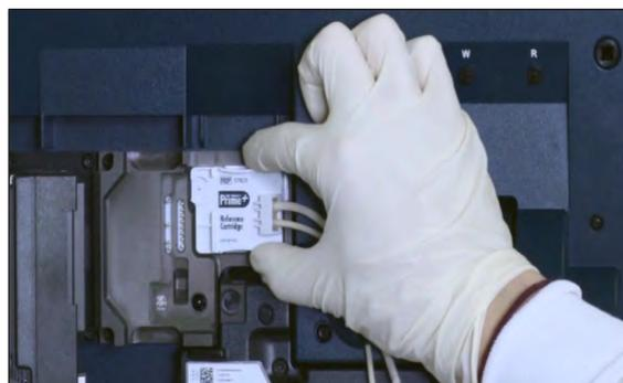
Figure 7.3 Reference Cartridge Removal
