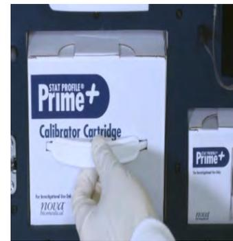
Figure 5.5 Remove Calibrator Cartridge
