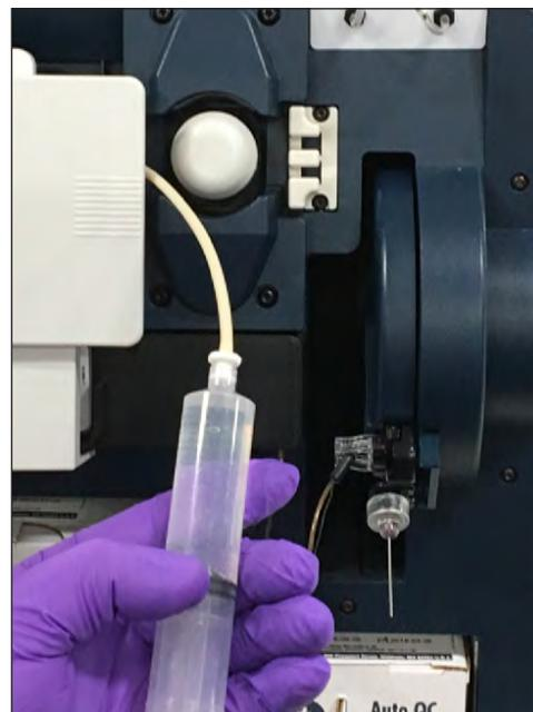
Figure 7.4 Tubing and 30-cc Syringe on Flush Tool
